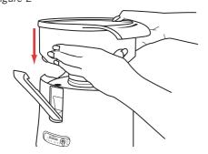
3. Position the stainless steel blade and filtering basket onto the motor drive shaft and push down until firmly in place, the arrows indicate the correct alignment position of the basket - figure 3.
